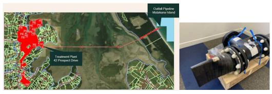
Figure 3-1 New Outfall 500m longer (L) and new Diffuser (2022) (R)
