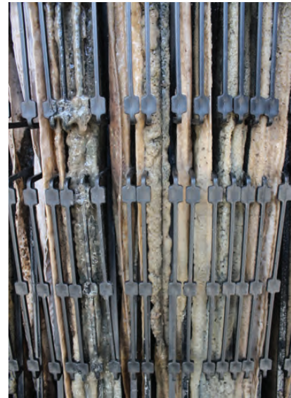
Suspended biomass vertically supported and surrounded by oxygen – a key feature of the BioGill technology.
